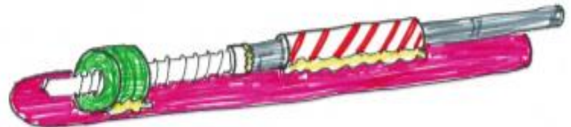
Glue threaded cap of glue stick to popsicle stick
